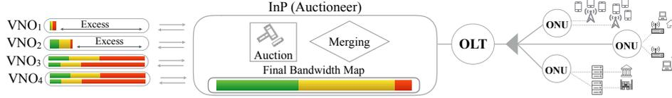
Fig. 1: Our proposed model for DBA capacity auctions in multi-tenant PONs.
